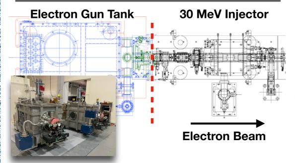
A replaceable electron gun unit with a tank for insulator oil was installed to minimize downtime of the facility (SP8 and SACLA).
