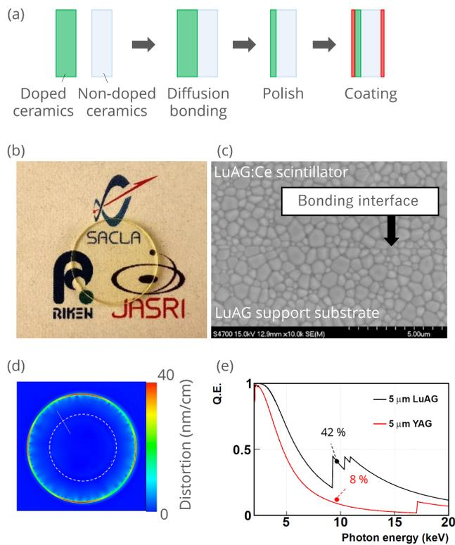
Fig. 1 (a) Fabrication process of thin-film transparent ceramic scintillators
