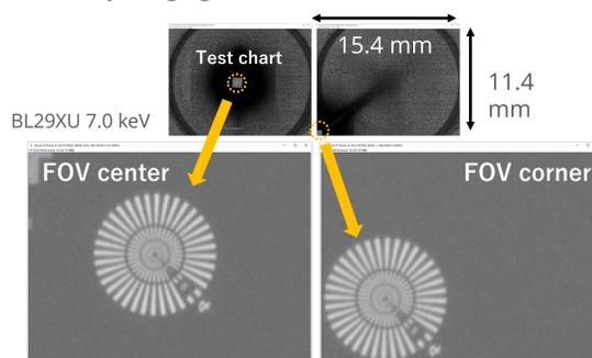
We are planning to develop a large-format X-ray imaging detector to enhance a field of view, implementing the SONY IMX411 image sensor. The prototype imaging unit has successfully visualized 1.2 μm L&S patterns in the center and the corner of FOV with 15.4 x 11.4 mm<sup>2</sup>.
