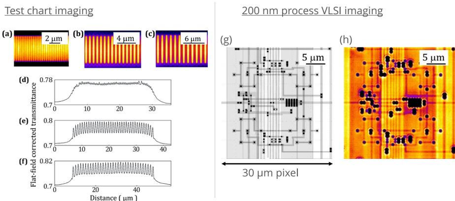
Fig. 3 (a-c) Transmitted X-ray images of 200/400/600 nm lines and spaces in the tungsten test chart
