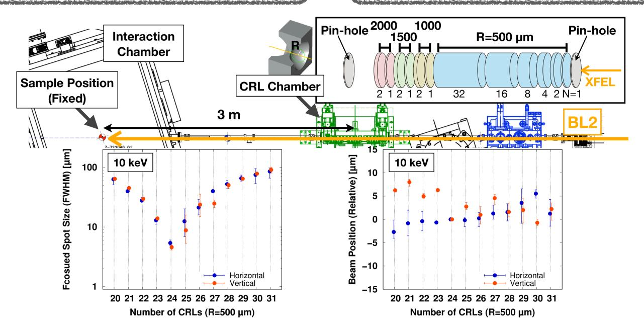
• In addition to the 2D focus by compound refractive lenses (CRLs), a 1D focus system using a mirror has been utilized. The system focuses the beam down to a few microns only in the vertical direction.
