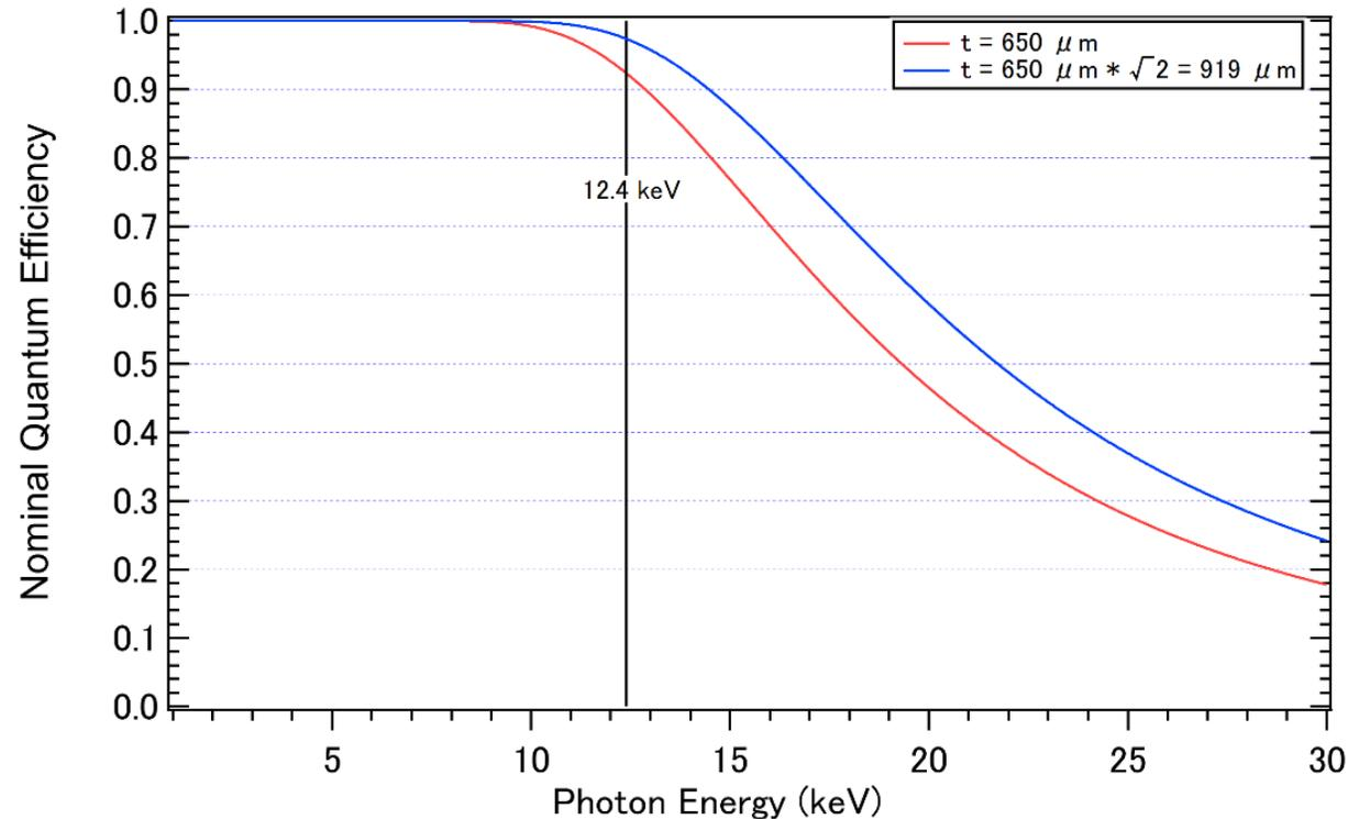
For CITIUS and MPCCD Phase III and III-L, Q.E. beyond 1 keV is well approximated by the thickness of silicon, where all the photons interacting Si through photo-electric effect are detected without loss.
