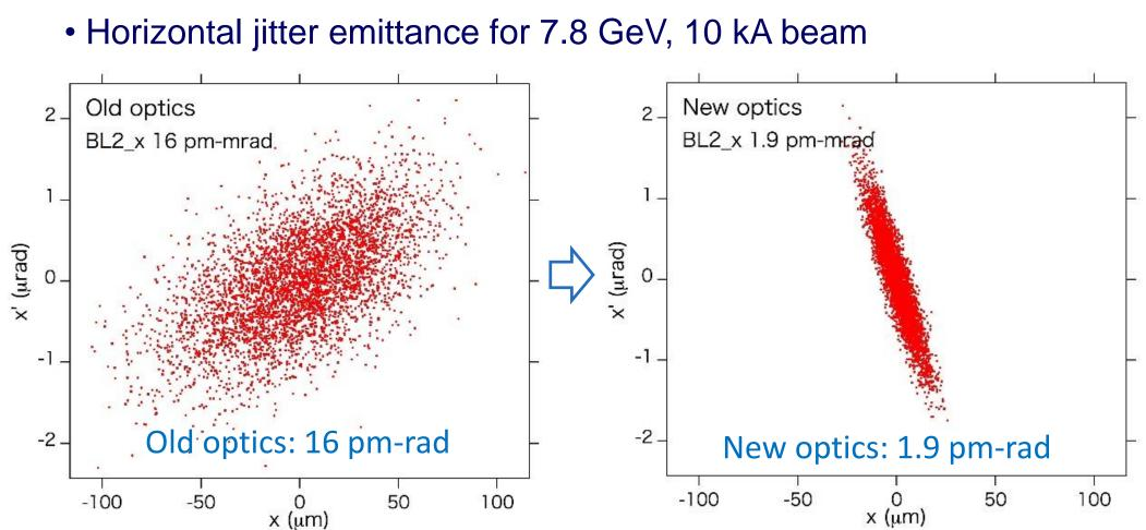
•Jitter emittance as a function of phase advance between two DBAs
