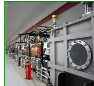
Themionic gun based low emittance injector
