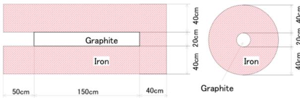
Figure 3 : Cut away view of the beam dump : the inner cylinder is made of graphite, the outer one from iron.
