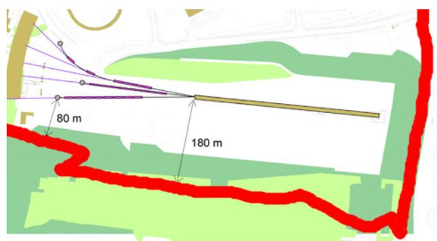
Figure 1 : Schematic view of the SCCS showing the closest distance between the loss points, the beam dump and the site boundary (in red).
