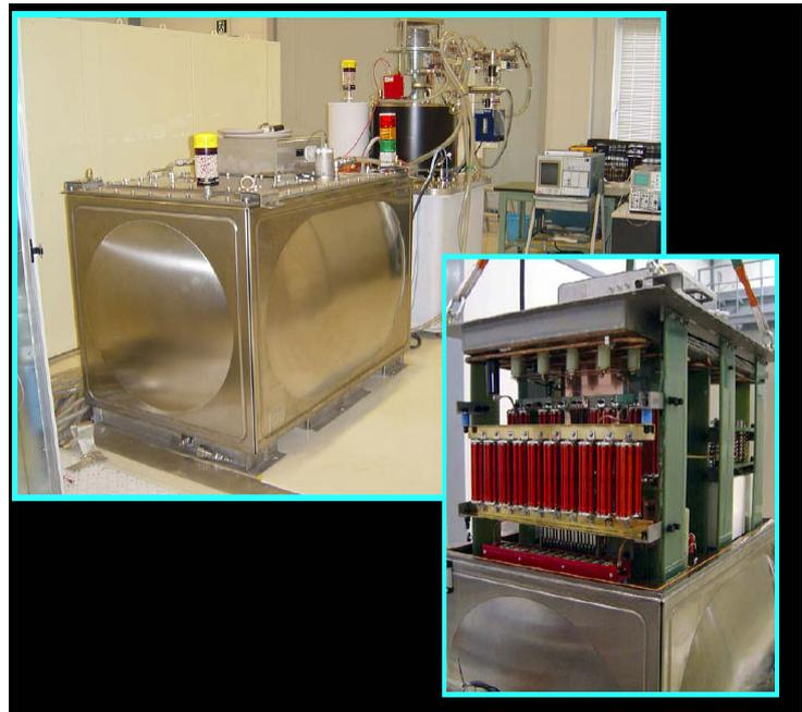
Fig. 3 Pulse modulator for 50 MW klystron and electron gu.
