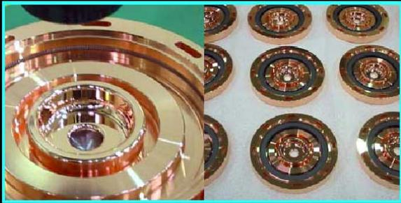
Fig. 6 C-band accelerating structure for SCSS. In each cell, the microwave absorber made by SiC was loaded to damp higher order modes.
