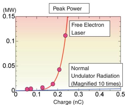
The peak power increases exponentially with the electron charge.
