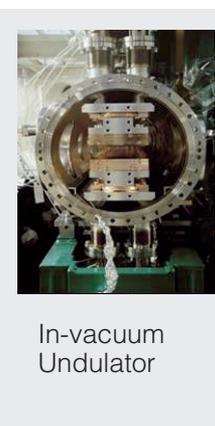
**The in-vacuum undulator generates strong XFEL radiation.**
